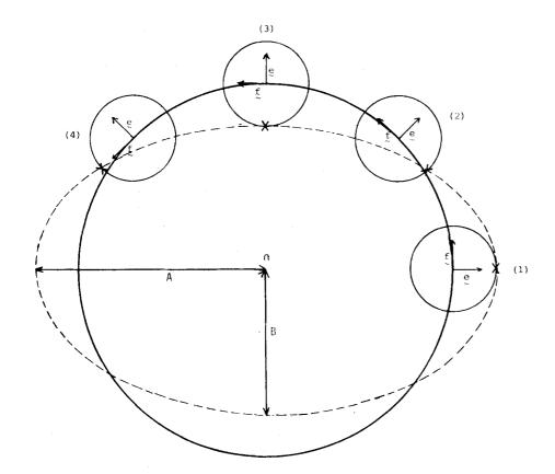
FIG. 1. Resolution of elliptical motion into two circular motions. The particle, whose position is marked X, rotates clockwise with angular frequency  $2\omega$  around the smaller circle, whose center moves anticlockwise with angular frequency  $\omega$  around the larger circle. Positions are shown at (1)  $\omega t = 0$ ; (2)  $\omega t = \pi/4$ ; (3)  $\omega t = \pi/2$ ; (4)  $\omega t = 3\pi/4$ .
