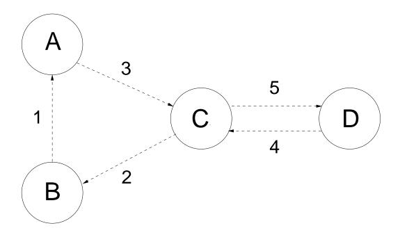
A packet switching network with 4 nodes (labelled A,B,C and D) and 5 links (labelled 1,2...,5)
