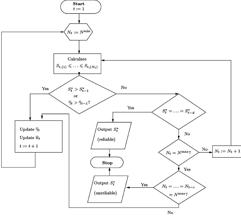
Figure 8. The flowchart for the FACE algorithm.
